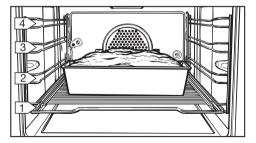
Place cakes in **rectangular tins** with the longer side across the width of the oven as shown, for optimum heat distribution and even results. Always use shelf level 1 for cakes in tins.
